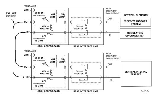
Figure 20. Insertion of VITS Test Signal
